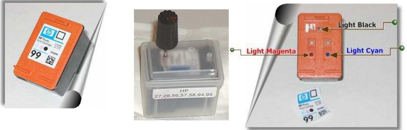
**Items needed: gloves, Photo/Light cyan, & Photo/Light magenta & Black Dye, hand-drill, #5 refill station, paper towels, review hints & tips and check list. Do not plug fill holes.**
