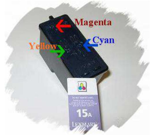
**Items needed:** gloves, hand-drill, #6 refill station, aluminum foil tape (located inside station # 4 in parts pack), cyan, magenta & yellow ink, paper towels, review hints & tips and check list **Note: Do not use the refill station lid for refilling this cartridge. Do not plug fill-hole. The regular version #15 is not refillable. The "A" version #15A can easily be refilled.**
